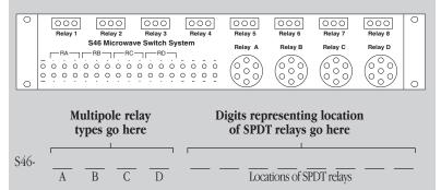
Multipole relay locations A - D: Enter a "3" for a SP3T relay, a "4" for an SP4T relay, a "5" for a SP5T relay, or a "6" for a SP6T relay in the required location. Enter a "0" in unused multi-pole locations. There must be digits in all four positions.
